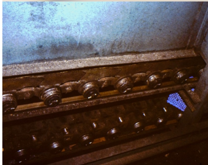
Any wear on the loaded side of the sleeve can be counteracted by turning the sleeve through 90° so as to present a new wear face.
